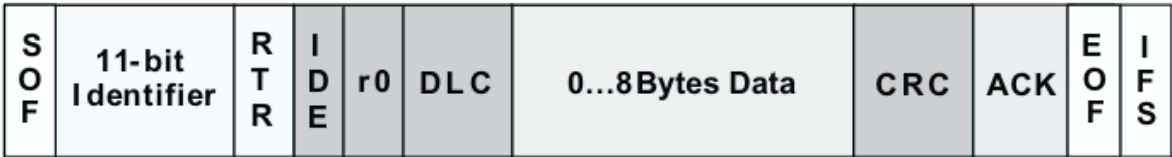
Figure 3. Standard CAN: 11-Bit Identifier
