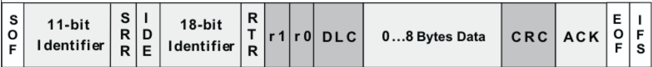
Figure 4. Extended CAN: 29-Bit Identifier
